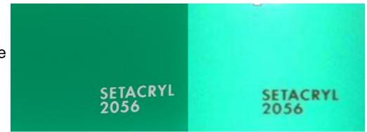
In this case we can notice that once the LED is on, the light source is visible through the sheet → spot effect
